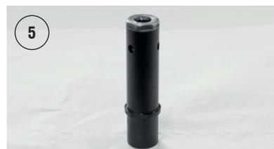
Position the gasket 8. Insert the assembly 2 to 8 into part 1. Reassemble the nosepiece according to the section «SETTING THE INSTALLATION KIT ON THE TOOL» p 5.
