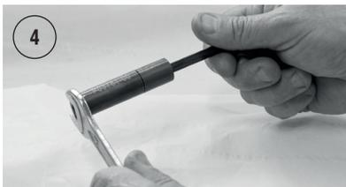
Then reassemble the whole. Screw piece 3 on the assembly 4 to 8. Tighten the whole assembly using the hexagonal wrench (6mm) provided and a 14mm wrench.
