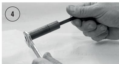
Then reassemble the whole. Screw piece 2 on the assembly 3 to 7: Tighten the whole assembly using the hexagonal wrench (6mm) provided and a 14mm wrench.
