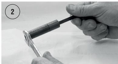
Separate the assembly 2 to 8 from the piece 1. Then unscrew part 2 from part 7 while holding the end of piece 2 with a SW wrench (14mm) and using the hexagonal wrench (6mm) provided.
