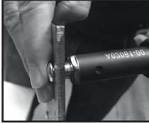
Insert completely the pin into the nose piece
