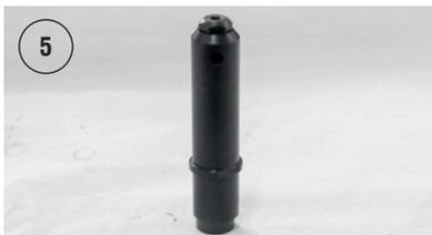
Insert the assembly 3 to 8 into part 2. Reassemble the nosepiece according to the section «SETTING THE INSTALLION KIT E-7-ACC-KIT5 ON THE TOOL» p 6
